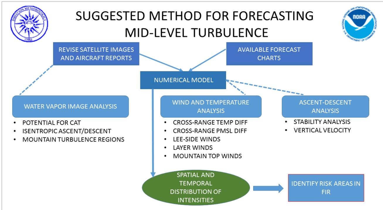
A method to forecast mid-level turbulence is proposed. It consists of revising satellite images and aircraft reports, and available forecast charts to then use numerical model output to issue a turbulence forecast. The forecast includes spatial and temporal distribution of turbulence intensities, which allow the identification of risk areas.
