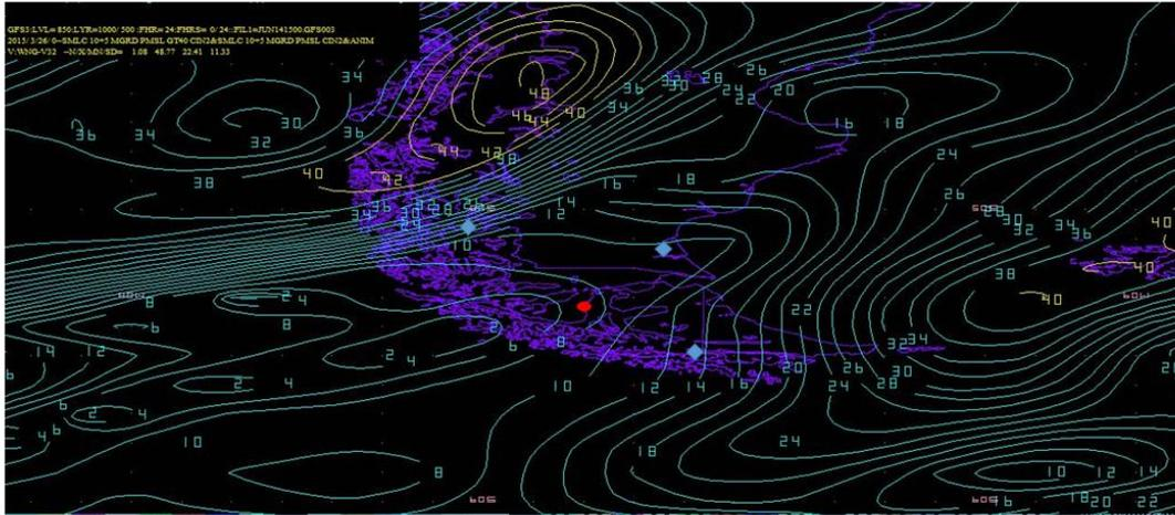
This slide contains an animation that is not visible on the PDF. The mean sea level pressure gradient provides an idea of the wind speed. This animation shows the evolution of large pressure gradients over/near SCCI.
