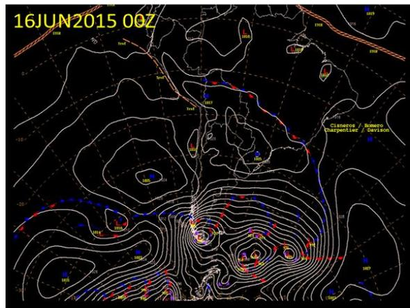
The South American Desk surface analysis shows the passage of the occluded low accompanied by a tight pressure gradient. The SCCI sounding shows speed shear between 800 hPa and 1000 hPa.
