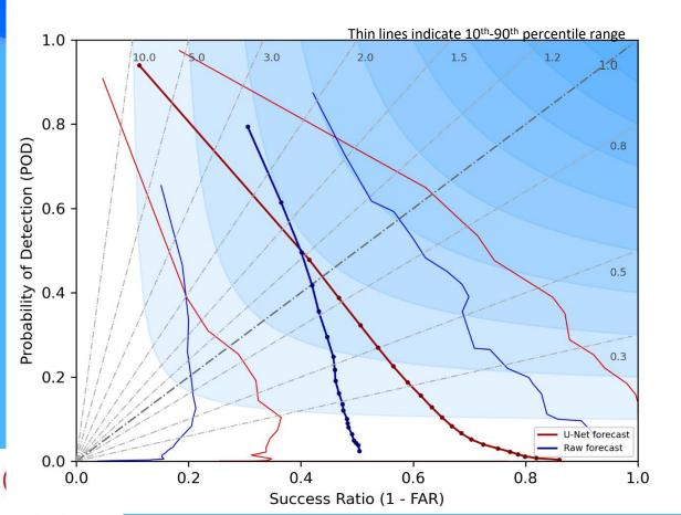
U-net ensemble performs comparably to or slightly outperforms raw NWP output from CAPS FV3 ensemble, depending on probability threshold.
